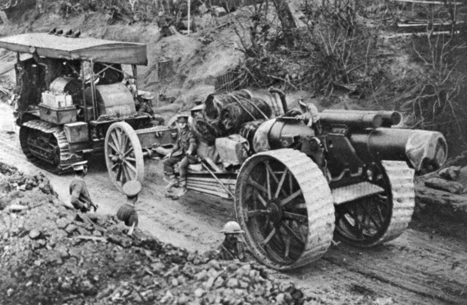
British Holt tractor towing a 8-inch Howitzer Mk V, 1916 – Author, U.K. government, public domain, Wikimedia
